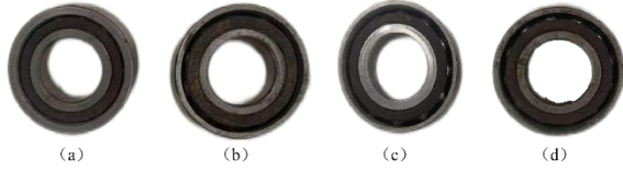
Figure 2. (a) Inner Ring Damage (b) Inner Ring Damage (c) Outer Ring Damage (d) Lack of Lubrication
