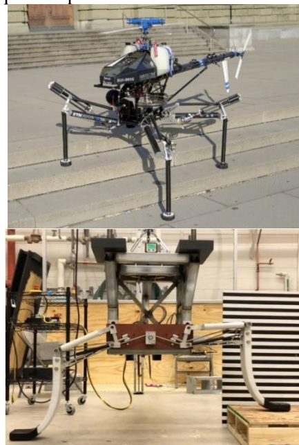
Figure 1. Bio-Inspired Passive Adaptive Landing Gear System.
